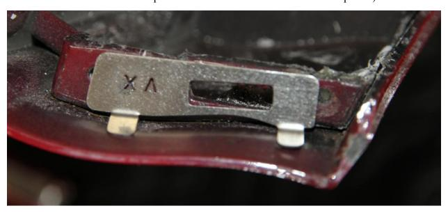
The plate includes tabs for extra stability and strength of the repair, so I bent those just slightly so that they were contacting the inside of the bumper cover. What does not show well in this photo is that the tab on the bumper is actually broken on the left side of the hole. So, this repair plate will provide a means to re-secure that tab in the original location and hold it firmly in place.
