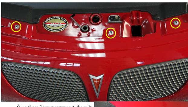
Once these 7 screws were out, the only thing left holding the bumper to the car are the tabs and brackets. In my case, I wanted to be particularly careful with the tab on the drivers side front, since that one is still OK on my GTO. The trick, if there is one, to try to protect these front tabs is to push on the bumper towards the rear of the car while, as gently as possible, pulling the bumper cover off the brackets. I was successful in removing the bumper without breaking anything.
